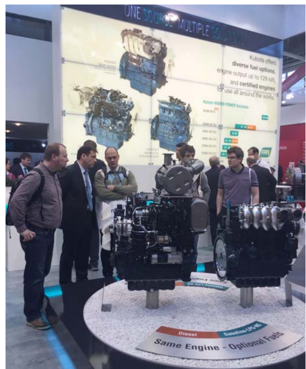
▲ Visitors scrutinize the technical details of a set of Kubota "twin footprint engines". On the left is the 86.4 kW model V3800-TIEF4B Kubota Diesel Engine while on the right is the 70kW model WG 3800 LPG Engine.
