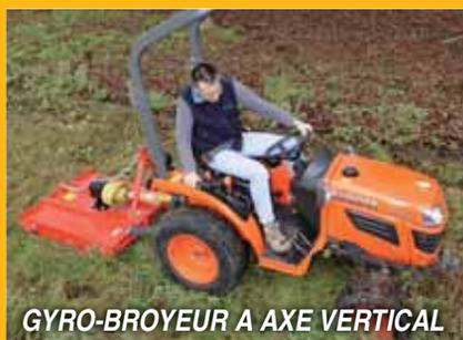
GYRO-BROYEUR A AXE VERTICAL
