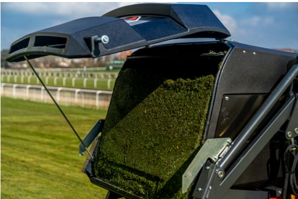
Chopped material transfer The powerful suction fan collects and dispatches chopped material quickly and effectively whatever the conditions. The clever design of the collector utilising a deflector inside, ensures the collector is filled completely every time to maximise the operation.
