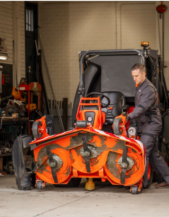
90° mower deck tilt. The mower deck can be tilted for any maintenance requirements. Quick, effortless positioning allows complete access to the underside.
