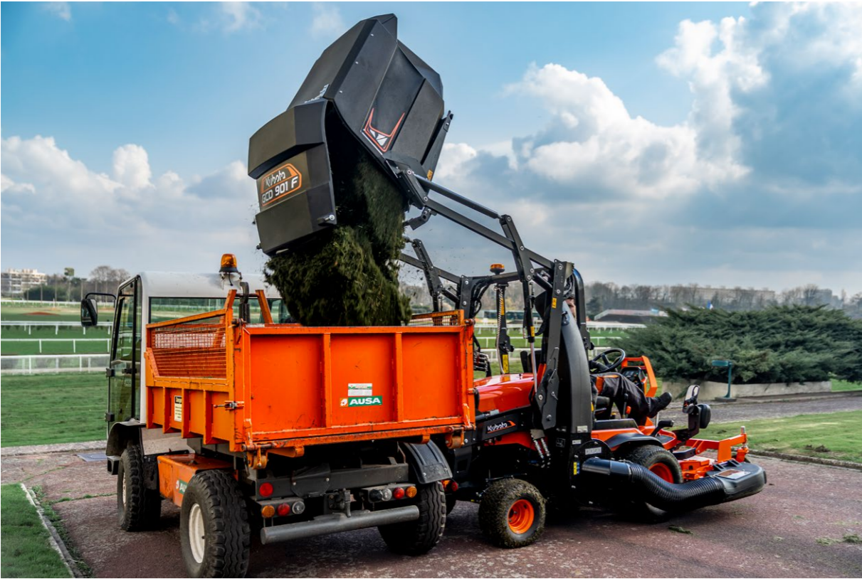
Large capacity collector A 700-litre capacity grass collector allows large areas to be worked before emptying. Lever operated, the high tip collector tank can be unloaded quickly and efficiently.
