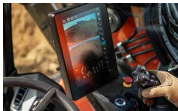
Height-adjustable premium joysticks and dual-display operating system
