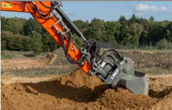
Hydraulic HS08 quick coupler with swivel unit
