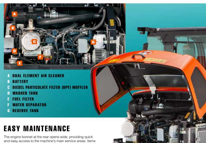
The engine bonnet at the rear opens wide, providing quick and easy access to the machine's main service areas. Items that require routine maintenance and service are within easy reach for fast and simple servicing. Quick-open panels on the right and left sides provide speedy access to the fuel refill (right side) and battery (left side). Other areas of the R070 and R090 are also easy to service and maintain.
