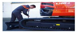
Wedge a steel tube into the track and turn the sprocket in the direction of reverse.
