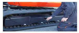
Apply a socket wrench on the nipple screwing adapter and loosen it slowly.
