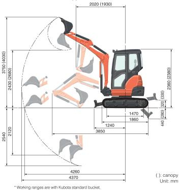
\* Working ranges are with Kubota standard bucket, without quick coupler.
