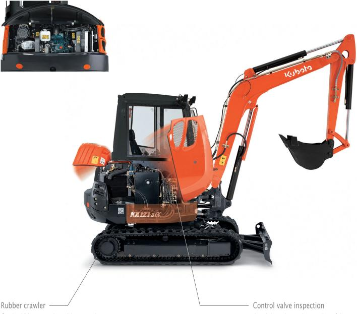
On the KX121-3 $\alpha$ , the rubber crawler design has better durability and stability when travelling. The lug pattern, with more ground contact surface and steel core positioning, are designed for better stability and less vibration when travelling. In addition, the double flange type track rollers contribute to better machine stability.
