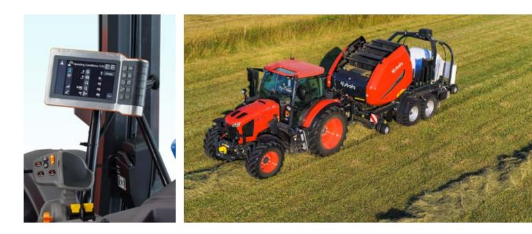
The proven, AEF-certified 7" K-Monitor is available as an option for the M6002. ISOBUS capability and an optional automatic steering system make the tractor ready for precision farming, enabling precise use of resources and efficient headland management.
