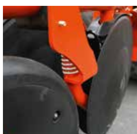
The Kubota CD-coulter consists of two steel discs (Ø410mm) with 12.5cm row spacing. Perfect depth control is ensured by the press wheels (Ø 380mm).
