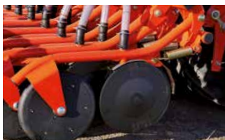
The Kubota CD-coulter consists of two steel discs (Ø410mm) with 12.5cm row spacing. Perfect depth control is ensured by the press wheels (Ø 380mm).
