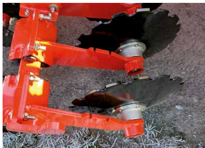
The first disc row ensures good penetration and prevents block-ages. The second row works offset and takes over the soil flow and plant residues of the first row.
