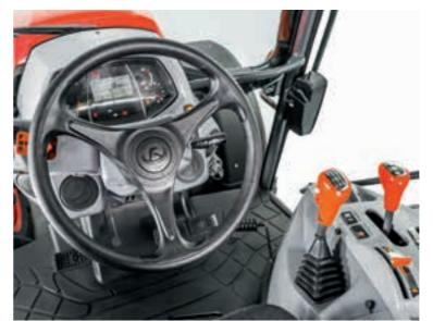
The handy steering wheel can be tilted forward when you exit the cab. Back in the seat, you can move it right back into its starting position. Simply press a pedal. Kubota has optimised the angle of the steering wheel, which gives you better visibility of the instrument panel and towards the front.
