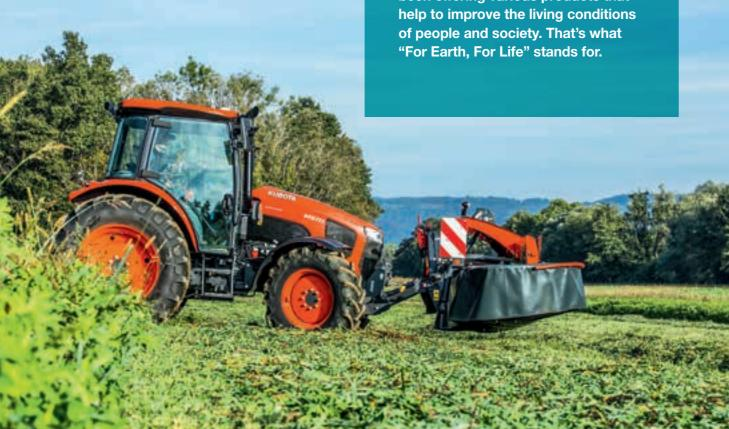
The front axle with bevel gear drive makes the M5001 extremely maneuverable, featuring a terrific 55° steering angle. This makes the tractor predestined for jobs in tight quarters. For over 30 years, Kubota has been using front axles with bevel gear drives. For good reason, as this combination is not only responsible for the very tight turning radius, but also allows for the elimination of the high-maintenance universal joints.
