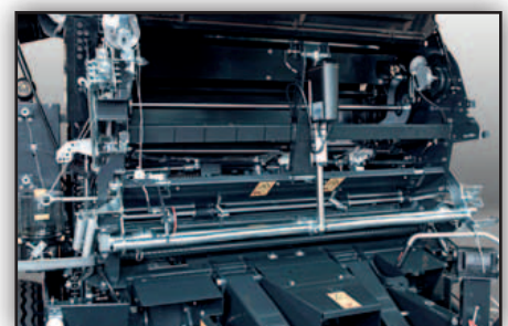
Twin tube fast operating twine binding system.
