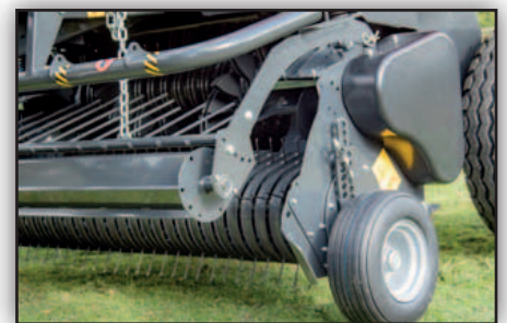
Pick-up guide wheels with generous flotation tyres. The unique pick-up drive design keeps the wheels within the overall baler width eliminating the need to remove them for transport.
