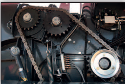
Main bale chamber drives are by heavy duty 1 1/4" pitch chain for a longer lifetime and reduced maintenance.
