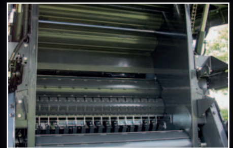
PowerMax Chamber: 17 heavy duty rollers for high density bale production.
