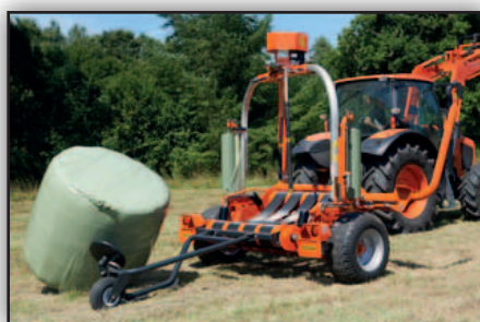
Kubota WR1850 can be fitted with a bale on end kit. The bale is tipped off gently without damaging the film wrap.
