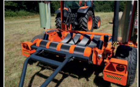
Wrapping table with belts and rollers.
