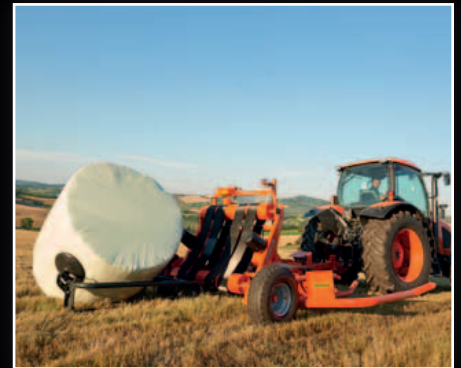
The Kubota WR1400 can be fitted with a bale on end kit. The bale is tipped off gently without damaging the bale.
