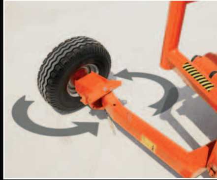
For narrow transport width, the right hand wheel is turned to the inside of the support arm.
