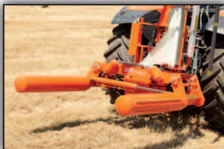
Easy and gentle self-loading of the bales – the bale is gently lifted by the rollers.
