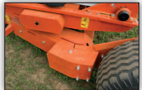
Extra counter weights can be fitted on the left hand side of the machine to ensure full stability also for the heaviest bales.
