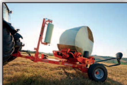
Low design of the machine ensures fast and gentle unloading of the bale with no need for a fall damper.
