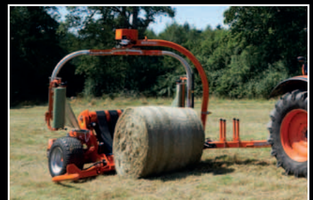
The bale is rolled onto the wrapping table for gentle handling.
