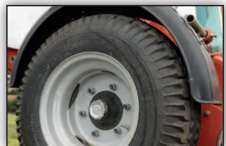
Mud guards reduce mud and dirt building up on the pre-stretcher and film rolls when operating in soft ground field and during transport.
