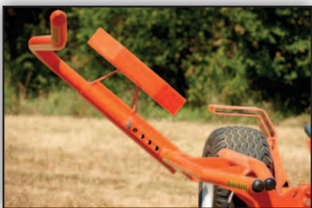
The adjustable loading arm with rear end stopper and inner support tube, allows the bale to be picked up and loaded on the move.
