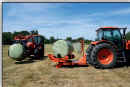
.. and pick up the already finished bale while the next one is being wrapped.
