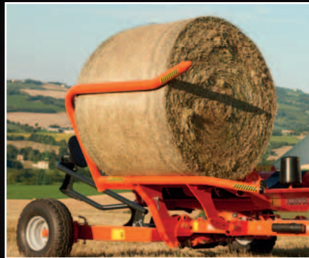
Hydraulically operated loading arm, with a low loading height, provides fast transfer of bale from arm to turntable.
