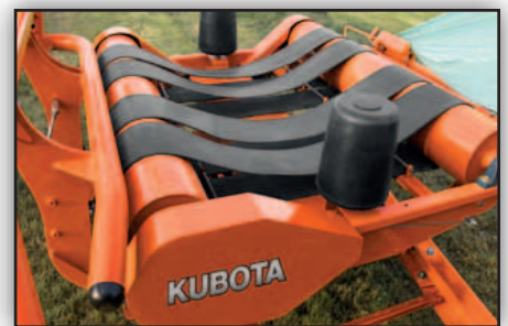
Turntable with two driven rollers designed for high bale stability and smooth even rotation.
