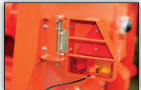
The Kubota BC1300 PRO and BC1600 PRO can be fitted with lighting kit, well protected from damages.
