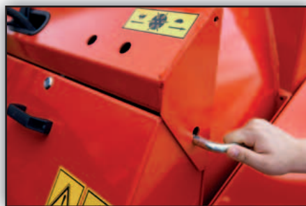
Easy shifting from bedding to feeding on the 2-speed gearbox.
