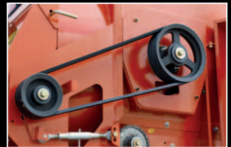
V-belt drive - low maintenance and quiet drive of the metering drum.
