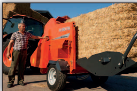
Operation of both tailgate and floor chain by using the remote control.
