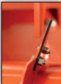
A patented system - the knives pass the fixed comb on alternative sides for a more even cut.
